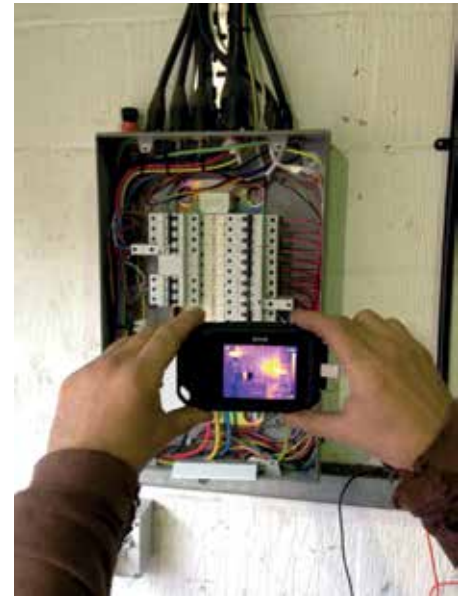
Gary Fisher: "With the FLIR C2, it's easy to see objects and heat areas clearly and with plenty of detail, which helps quickly identify the areas that need attention."
