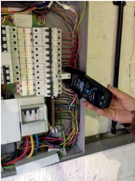
The FLIR CM174's narrow clamp jaws help getting in between all the cables inside consumer units.
