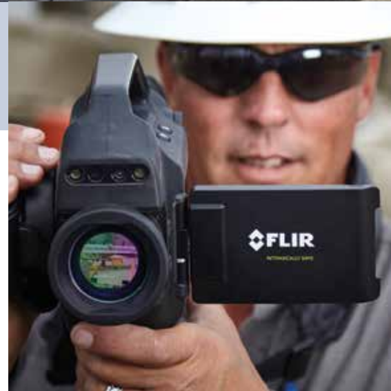
The FLIR GFx320 OGI camera visualizes most hydrocarbons used in the oil and gas industry, and carries an Intrinsic Safety designation
