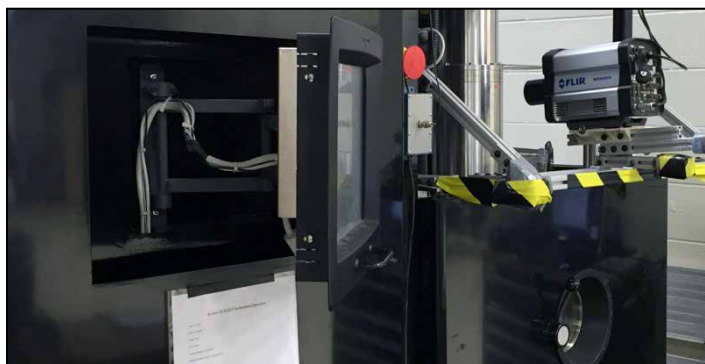
FLIR SC8202 MWIR camera monitors a stage of the AM process.
