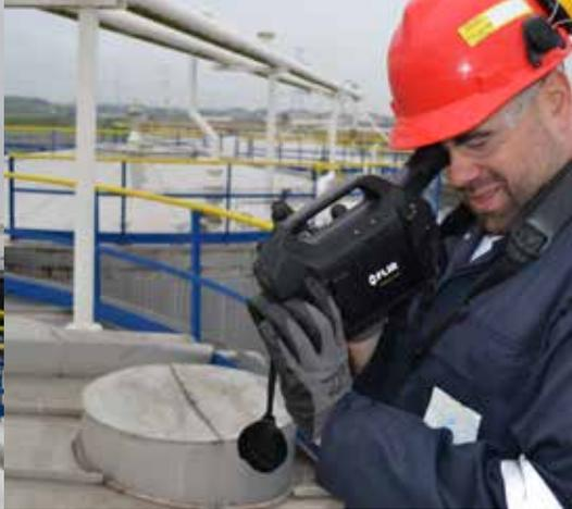
Bart Segers: "The FLIR GFx320 is easy to carry, much lighter than any optical gas imaging camera I have worked with, and also much more comfortable than the usual TVA probe gear that you have to carry around, especially when you're on site for an entire day."
