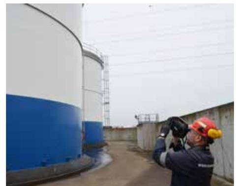
Bart Segers, The Sniffers: "With the GFx320, you can monitor large areas from a safe distance. You can get an overview of the entire target without having to build scaffolds."
