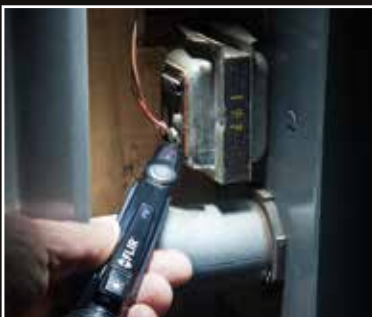
High sensitivity mode is useful for working on low-voltage systems
