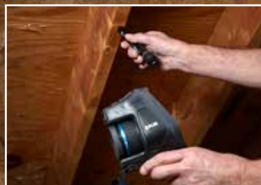
Use MR40 to confirm whether the cold spot found in a thermal image is moisture
