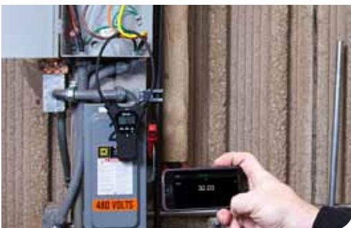
The CM57's bluetooth capability gives readings at safe distances
