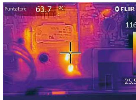
*Thermal image of the electronic circuitry of an oscilloscope, with MSX*
