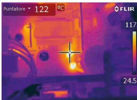
*Thermal image of the electronic circuitry of an oscilloscope*
