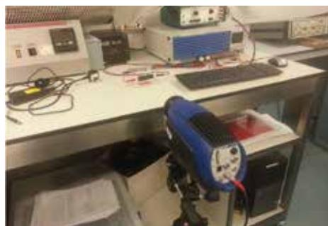
FLIR SC5000 camera in operation looking at a 18650 battery
