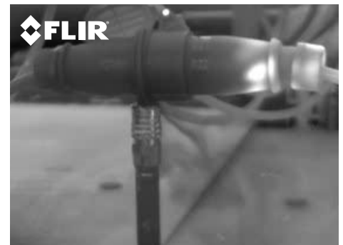
The FLIR GF320 visualises invisible gases at leak sites as dark plumes of smoke.
