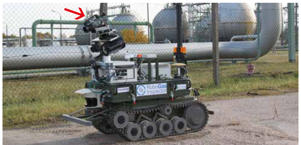
The RoboGas Inspector consists of three modules: a chain-driven mobile platform, a navigation module and an inspection module. Note the FLIR GF320 on top of the unit.
