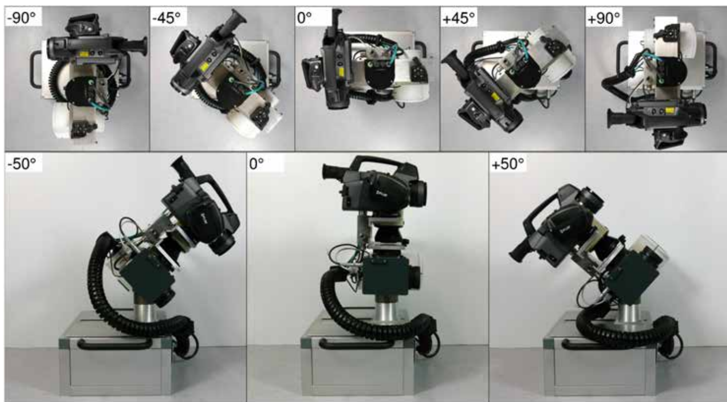
Panning range (view from above) and tilt range (side view from below) of the sensor system
