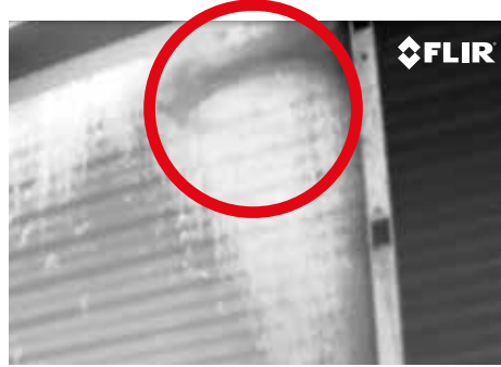
A refrigerant gas leak in visual video, thermal video and thermal video in High Sensitivity Mode (HSM)
