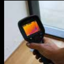
Find air infiltration problems
