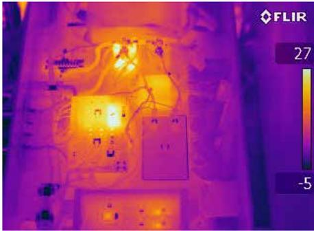
Electronic battery box under load
