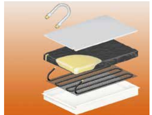
The MeandRo system used consists of perforated sheet steel ceiling panels in a sandwich construction, factory-equipped with a MeandRo element.
