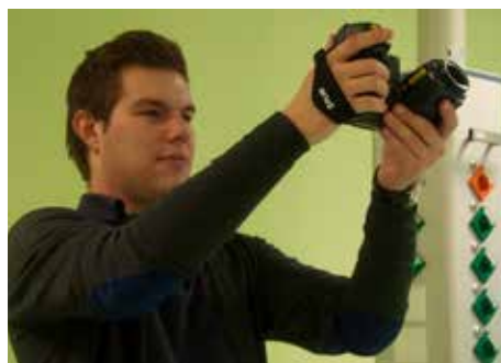
De FLIR T400bx series is equipped with a tiltable optical unit that allows for picture-taking from every desired angle with a comfortable work posture.
