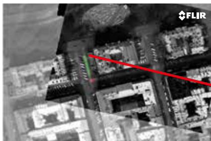
After seeing this leak in the report, the district heating company went there to investigate. It turned out to be a very large leak. Needless to say the company was very glad that this major leak was detected.
