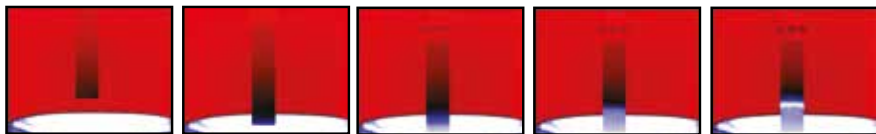
This sequence of thermal images shows the wicking test result for a woven mesh made of stainless steel.
