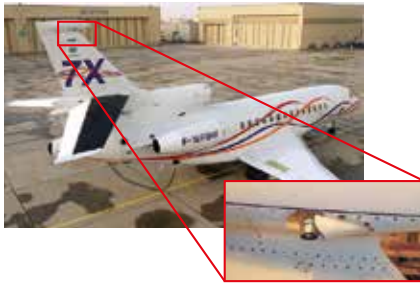
The FLIR thermal imaging camera was mounted in the top of the tail of the Falcon 7X, looking down on the right horizontal stabilizer.
