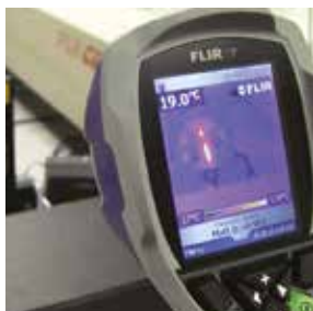
The heat from invisible infrared laser beams clearly shows up in the thermal images. By visualizing the heat from infrared laser beams FLIR helps to guarantee the researchers' safety.
