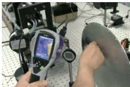
Using the FLIR thermal imaging camera Ma aligns the optics in his research setup.
