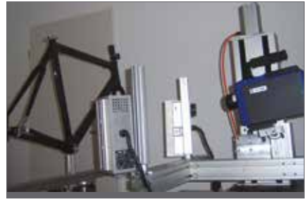
The bike frame is mounted on a rotary table.
