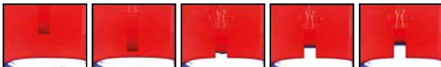
This sequence of thermal images shows the wicking test result for a porous glass frit.
