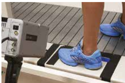
The thermal imaging camera finds the hot-spots on the ClimaCool™.
