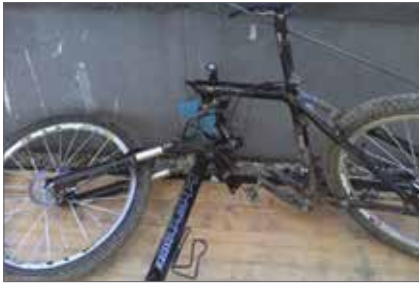
This is what might happen to a carbon fiber based bike frame if defects remain undetected.
