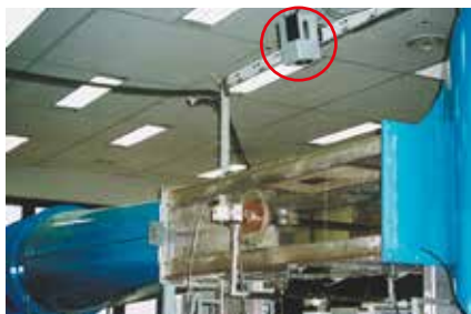
The wind tunnel with the FLIR thermal imaging camera
