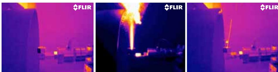
The ASTM- G175 test investigates the ignition sensitivity of oxygen components to a promoted ignition impact. Ignited material is blown into the oxygen component and the thermal sequence is used to determine how strongly the component reacts.
