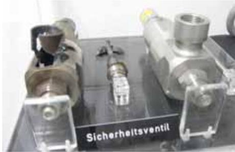
This valve showed a devastating positive feedback loop during an oxygen pressure shock test which consumed the valve in the process. Needless to say the client discarded it as a flawed design.
