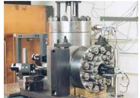
Test apparatus for determining the combustion behavior of metallic materials in high pressure oxygen - the test setup will include the FLIR thermal imaging camera in the near future with the inclusion of an infrared window.
