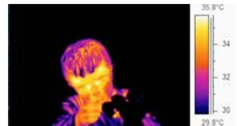
Small temperature differences in facial regions can be used to monitor autonomic responses of human test subjects without applying contact sensors or otherwise impeding the movement of the test subject.
