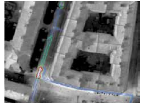
The thermal images are analyzed and an extra layer of information is added. District pipelines are marked with blue lines. Green outlines mark smaller leaks and red outlines mark serious leaks that require immediate attention.
