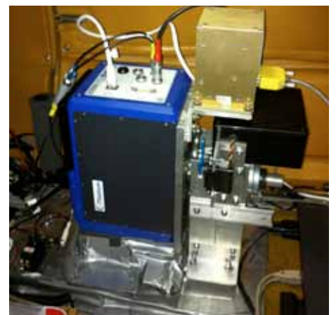
A gyro-stabilized platform compensates for the plane's movements, enabling the FLIR SC7600 thermal imaging camera to record steady thermal images.
