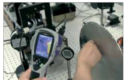
Using the FLIR i7 thermal imaging camera Ma aligns the optics in his research setup.
