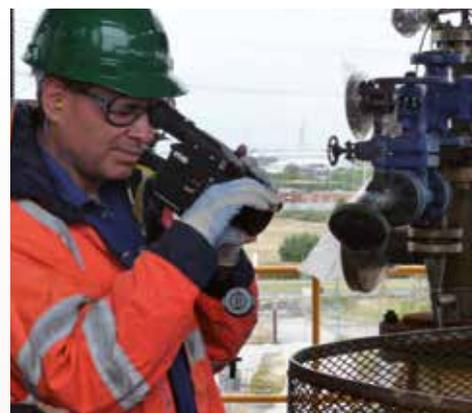
Dave Fashimpaur from BP is checking for leaks of natural gas using his GasFindIR HSX
