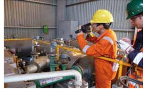
*In both pictures CO leaks were found with the GasFindIR CO*
