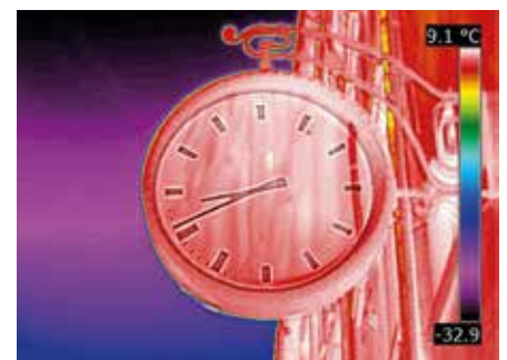
Thermal image now using the MSX-setting. Note that more details are visible.
