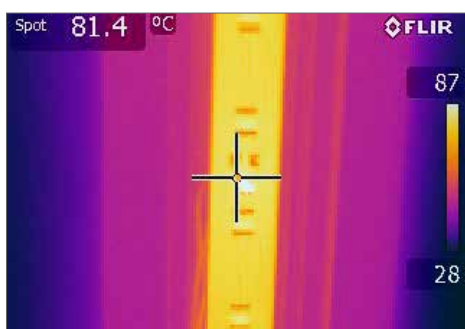
Temperature measurement of an LED board
