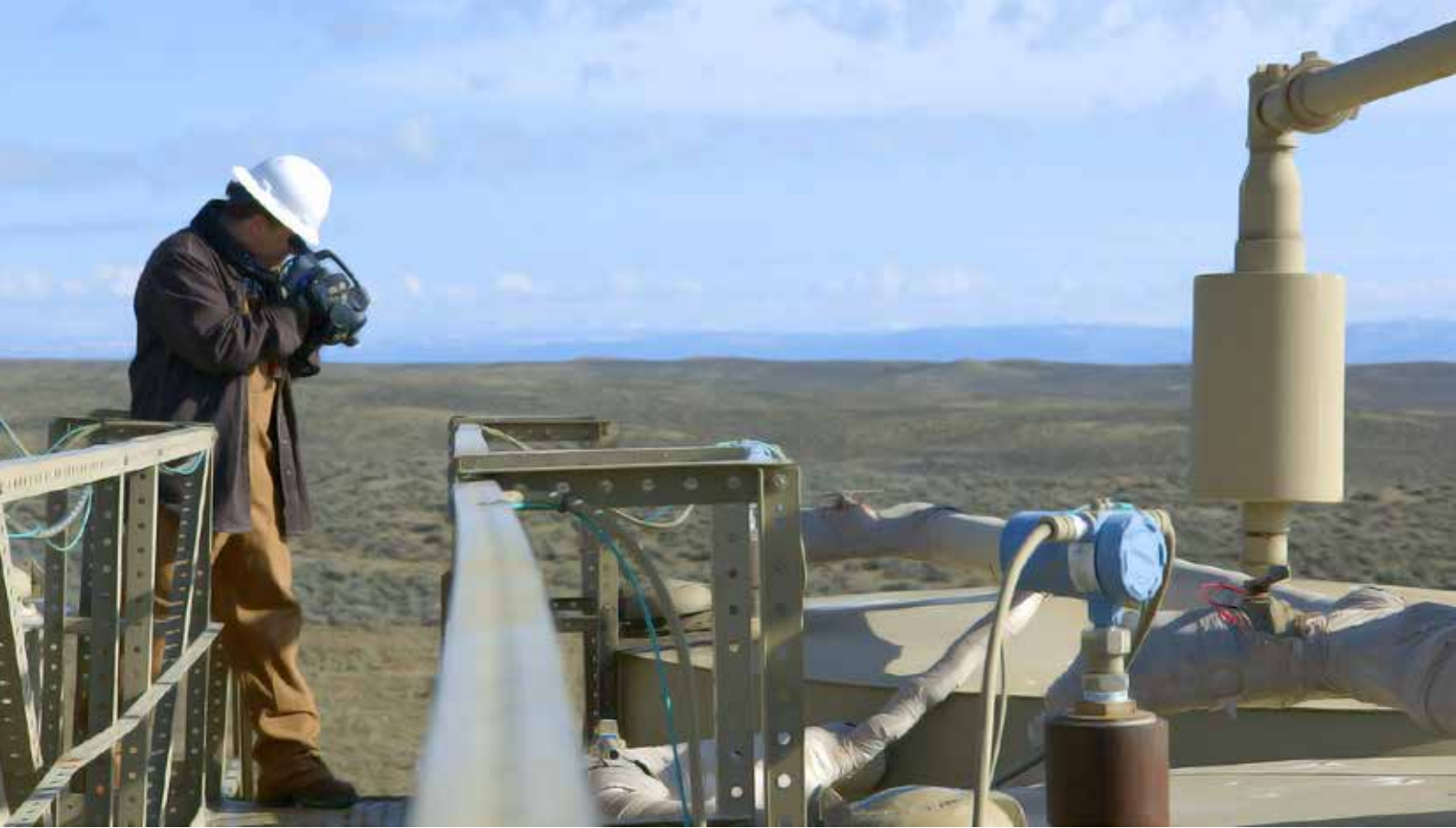
Optical gas cameras can scan areas that are impossible to reach with TVAs
