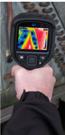
FLIR E4: temperature measurement in 4,800 spots
