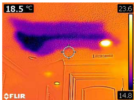
HVAC condensate overflow soaks a ceiling
