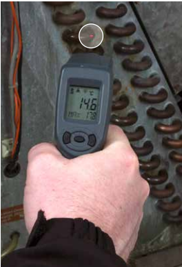
IR thermometer: temperature measurement in one spot
