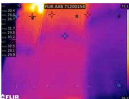
Cast resin transformers need to be able to handle temperature shocks safely. Insulation breakdown on cast resin transformers can lead to system failure and safety issues. The FLIR AX8 can detect temperature raises due to insulation breakdown in an early stage.
