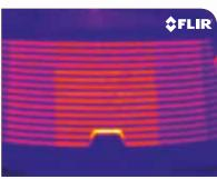
Inspection of a windshield defroster for damaged electrical elements.
