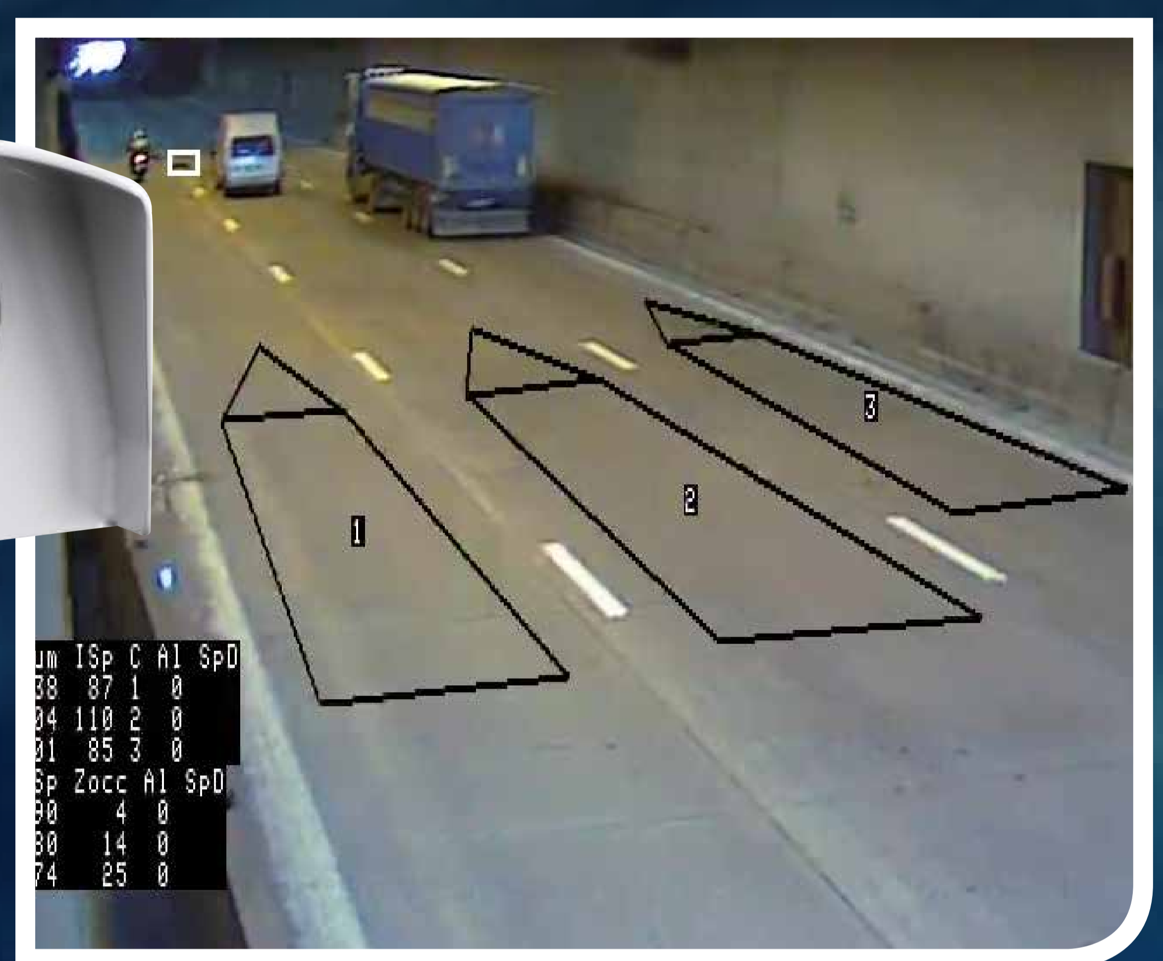
Automatic Incident Detection
