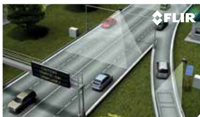
TrafiCam x-stream is an above-ground sensor providing a wide range of traffic data on up to 4 lanes.
