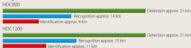
Actual range may vary depending on camera set-up, environmental conditions, user experience and type of monitor or display used. Assumptions: 50% probability of achieving objective at specified distance given approximately 2°C temperature difference and 0.82 / km atmospheric attenuation factor. DRI according to Johnson Criteria.
