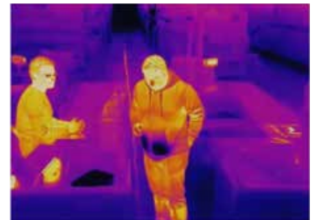
The XPredator anti-theft system works on the principle of heat energy coming off the environment and looks for heat differences between the stolen goods and the rest of the human body.
