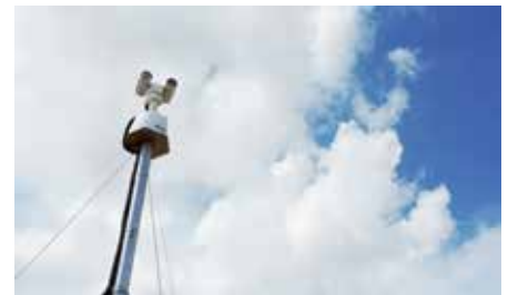
Whenever a target is picked up by the radar, the automatic slew-to-cue mechanism of the FLIR PT-602CZ pan/tilt camera is activated.
