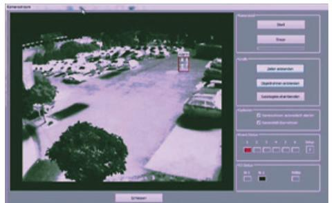
*The video analysis method used here was specifically aligned with thermal imaging technology: If somebody gets into the secured area an alarm is being processed.*
