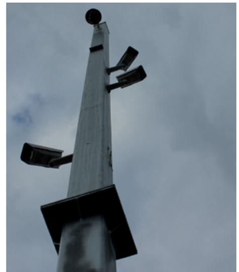
Three FC series S FLIR cameras monitor different areas from a central mast and, in the case of an alarm, they trigger a central high-speed dome camera to identify the perpetrator.
