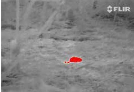
The squirrels are easy to spot thanks to the InstAlert™ feature, which colors the hottest part in the thermal image red, available on all FLIR Scout PS-Series.
