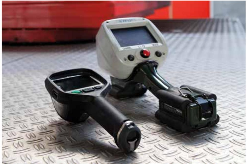
FLIR K50 next to the FireFLIR. Although the FLIR K50 is the preferred tool due to its compactness, the FireFLIR is still proving its worth after 10 years and is still in operation. It was extensively used during the fire at the Kalmthout Heath in 2011.
