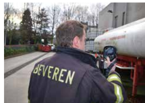
With the FLIR K50 you can see temperature changes resulting from all kinds of chemical reactions in containers, something that is very useful to the Beveren fire department because of the many chemical industry companies in the Waasland port.
