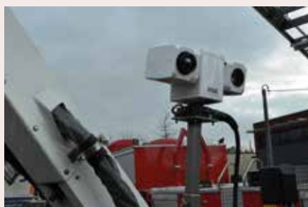
The Beveren fire department uses a PTZ system with a visual and a FLIR thermal camera to monitor fire situations.
