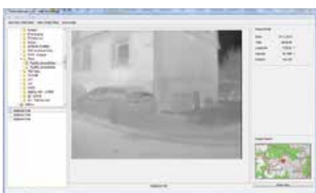
The ThermoViewer software reads the raw data from the USB and converts it to black & white or color images.
