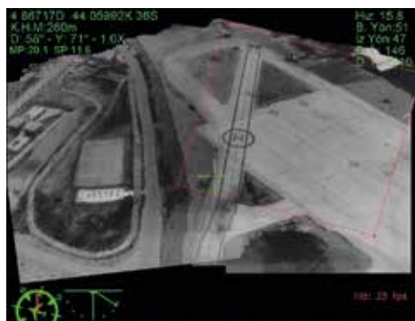
The mosaic software is stitching consecutive images as the camera turns or as the UAV moves, providing a broader situational awareness.
