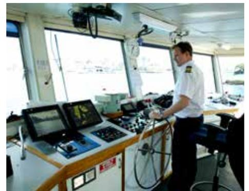
The joystick is on each bridge console, as close to the wheel as possible, so all features are right at the master's fingertips.
