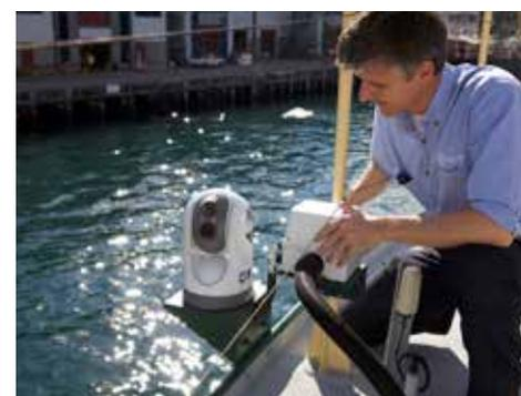
*The compactness of the M-Series thermal imaging cameras allowed them to be accommodated within real estate constraints of what was already fitted to each vessel.*
