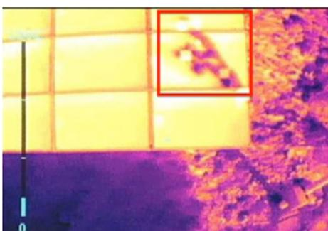
The combined use of thermal and visible data allows recognizing for example the effect of a shadows. The red square indicates the shadow of a pole in the plant.
