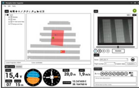
A screenshot of the Solar Inspector running on a Windows 8 tablet PC. The red area on the left corresponds to the image shown on the right.
