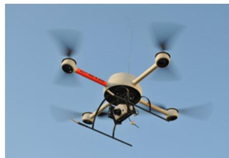
*mT-Panoptes includes a FLIR TAU 640 thermal core and a 720 p video-camera. It comes with a carbon fiber cart which allows mounting underneath small drones.*
