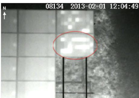
Thermal images taken from different heights (about 10 m in the left image and 20 m in the right). Hot cells in modules are evidenced by red circles.
