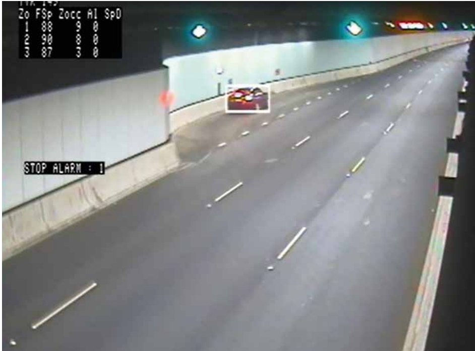
The FLIR video server can detect a wide range of incidents, including stopped vehicles.
