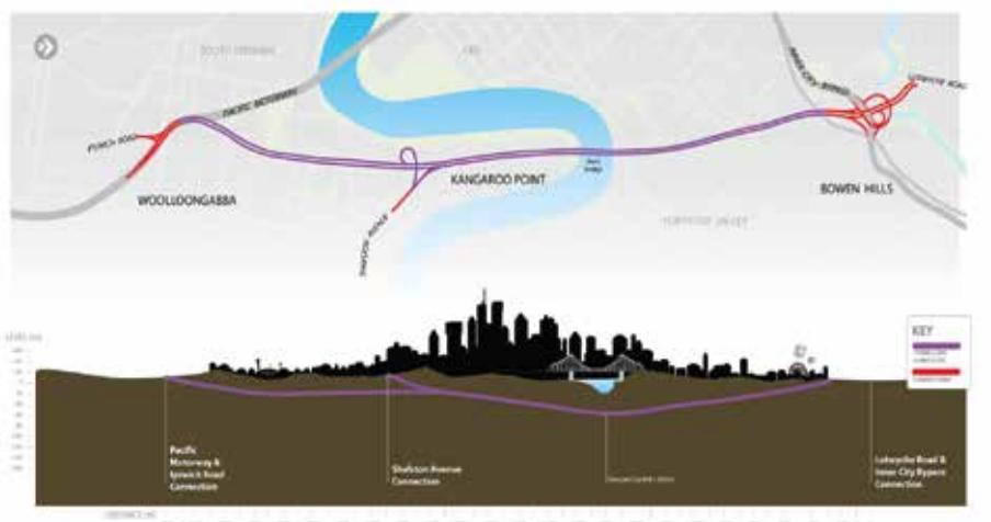
Alignment of the CLEM7 (in purple) with the different connections (in red). Next to the 5 existing connections, a sixth one will be added in 2012 with the new Airport Tunnel (on the upper right).
