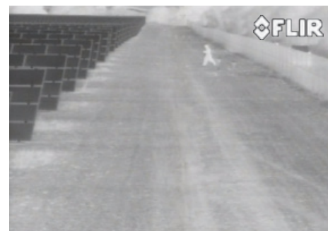
When the microwave intruder detection system is triggered the nearest FLIR PT-313 thermal imaging camera is automatically pointed towards the location where the alarm was triggered to verify the alarm.
