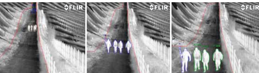
These thermal images are taken with a FLIR SR-324 thermal imaging camera, which has a 19 mm lens and a field of view of 24°. The distance at which these thermal images were taken is approximately, from left to right, 110, 40 and 10 meters.
