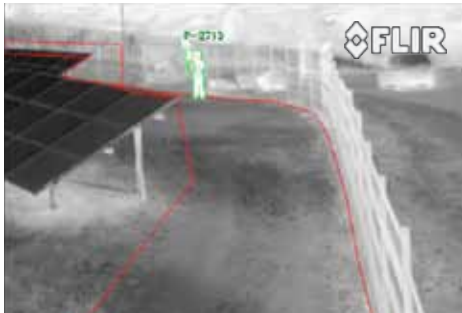
A fence alone is not enough to keep intruders out. Fences can be climbed quite easily. Thermal imaging cameras will help detect intruders before any property is damaged.
