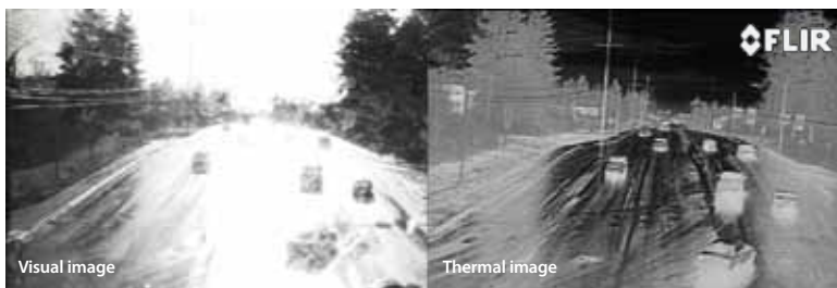
Thermal imaging cameras see through glare and back-lighting, improving signal control.
