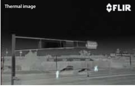
Thermal imaging cameras can see cars at the stop bar and pedestrians at the intersection clearly in the dark.
