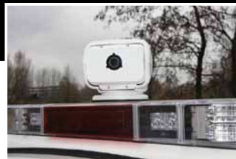
The FLIR PathFindIR thermal imaging camera is mounted in a pan and tilt platform for a searchlight.
