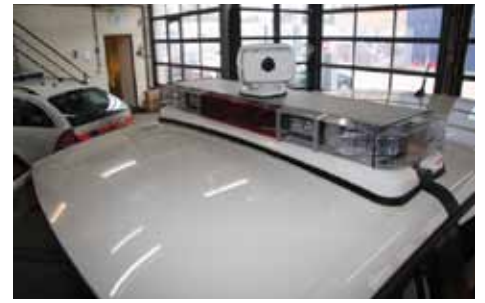
The FLIR PathFindIR is easy to integrate in the electrical system of the patrol cars due to its compact and lightweight build and economic energy consumption.
