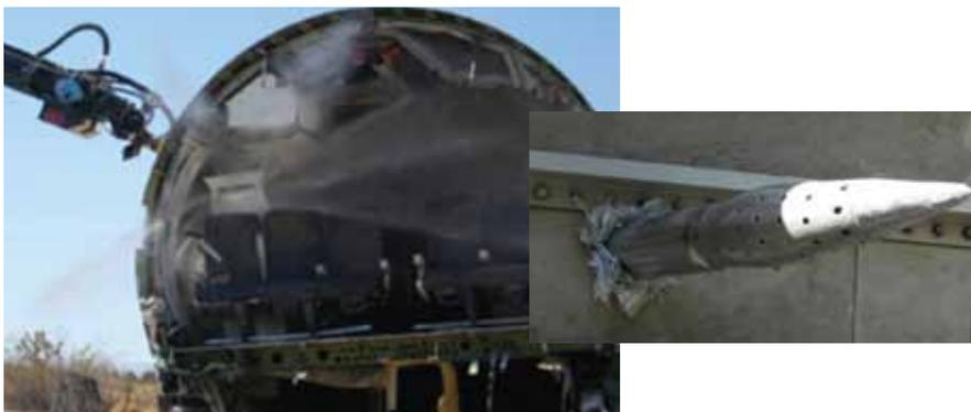
*This test shows that the Stinger's piercing tool can puncture an aircraft's hull from every possible direction. Jungmair: "That makes the Stinger really unique."*
