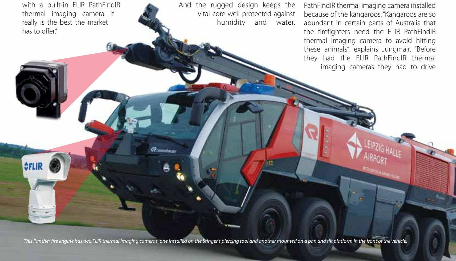
This Panther fire engine has two FLIR thermal imaging cameras, one installed on the Stinger’s piercing tool and another mounted on a pan and tilt platform in the front of the vehicle.
