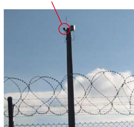
The FLIR Systems SR-100 is mounted on a pan/tilt together with a CCTV camera. The system is mounted on existing poles along the runway.
