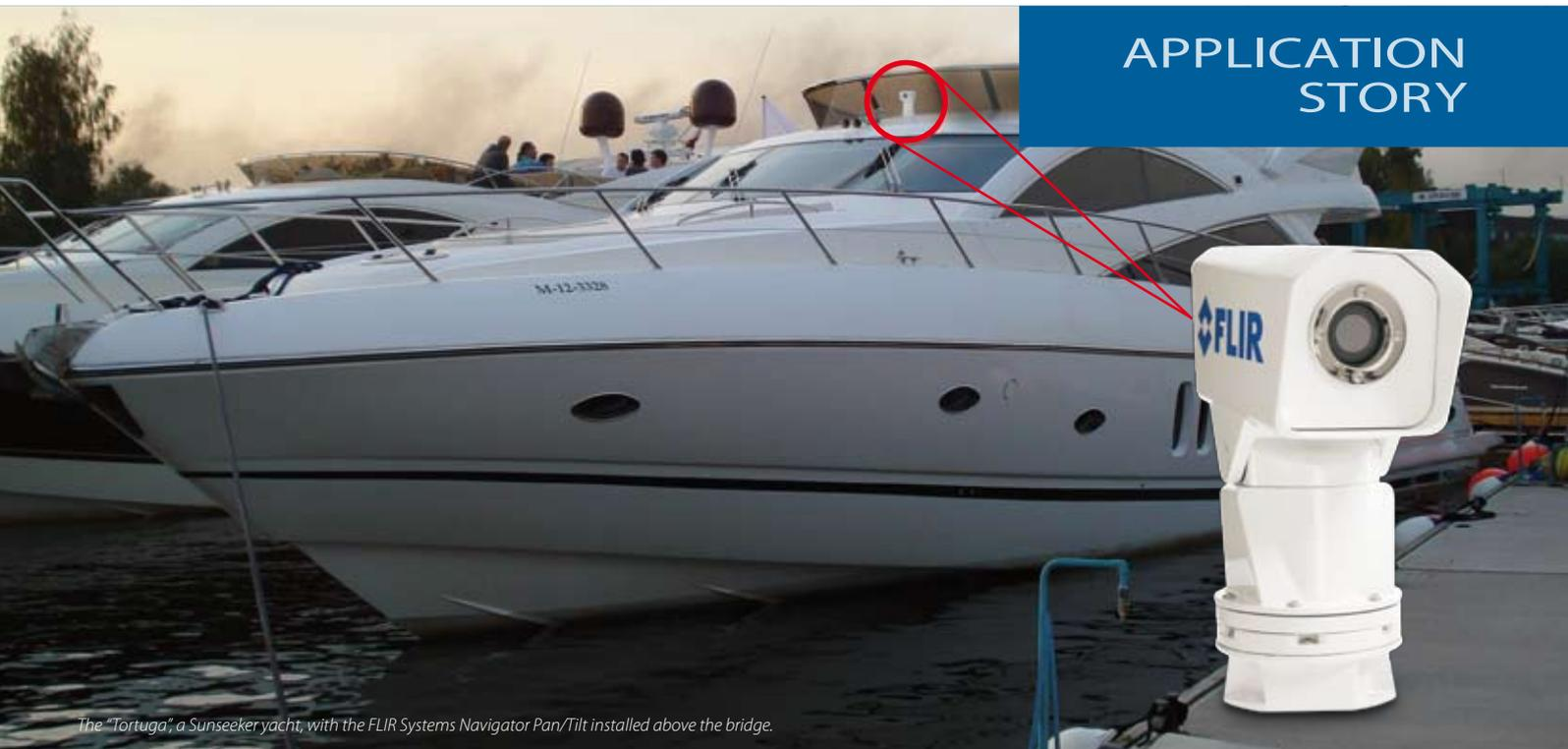
The "Tortuga," a Sunseeker yacht, with the FLIR Systems Navigator Pan/Tilt installed above the bridge.
