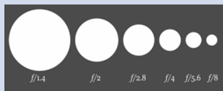
A lens with a higher f/number has a smaller diameter
