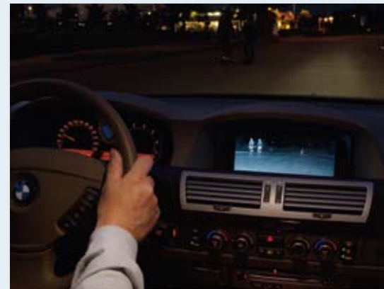
BMW opted for thermal imaging cameras with Vanadium Oxide detectors for their driver vision enhancement system
