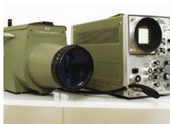
The first thermal imaging cameras were bulky systems that needed to be filled with liquid nitrogen
