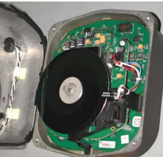
A ferroelectric detector has a continuous rotating chopper which is susceptible to breakdowns.
