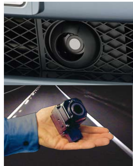
The size of a thermal imaging camera is an important factor if the camera needs to be integrated in confined spaces such as cars.
