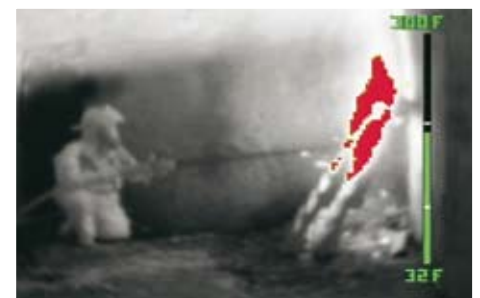
Not having a Thermoelectric Cooler is a big advantage in firefighting applications, since cameras are turned on and off to conserve battery power and any delays in producing an image can be potentially dangerous.
